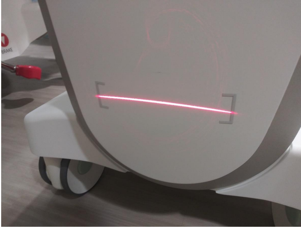
Figure 3: Close up view of positioning laser. The laser is designed to be centered within the confines of the small box on the front of the Bravos afterloader. This allows for an easy visual reference to ensure that CamScale positioning is correct.
