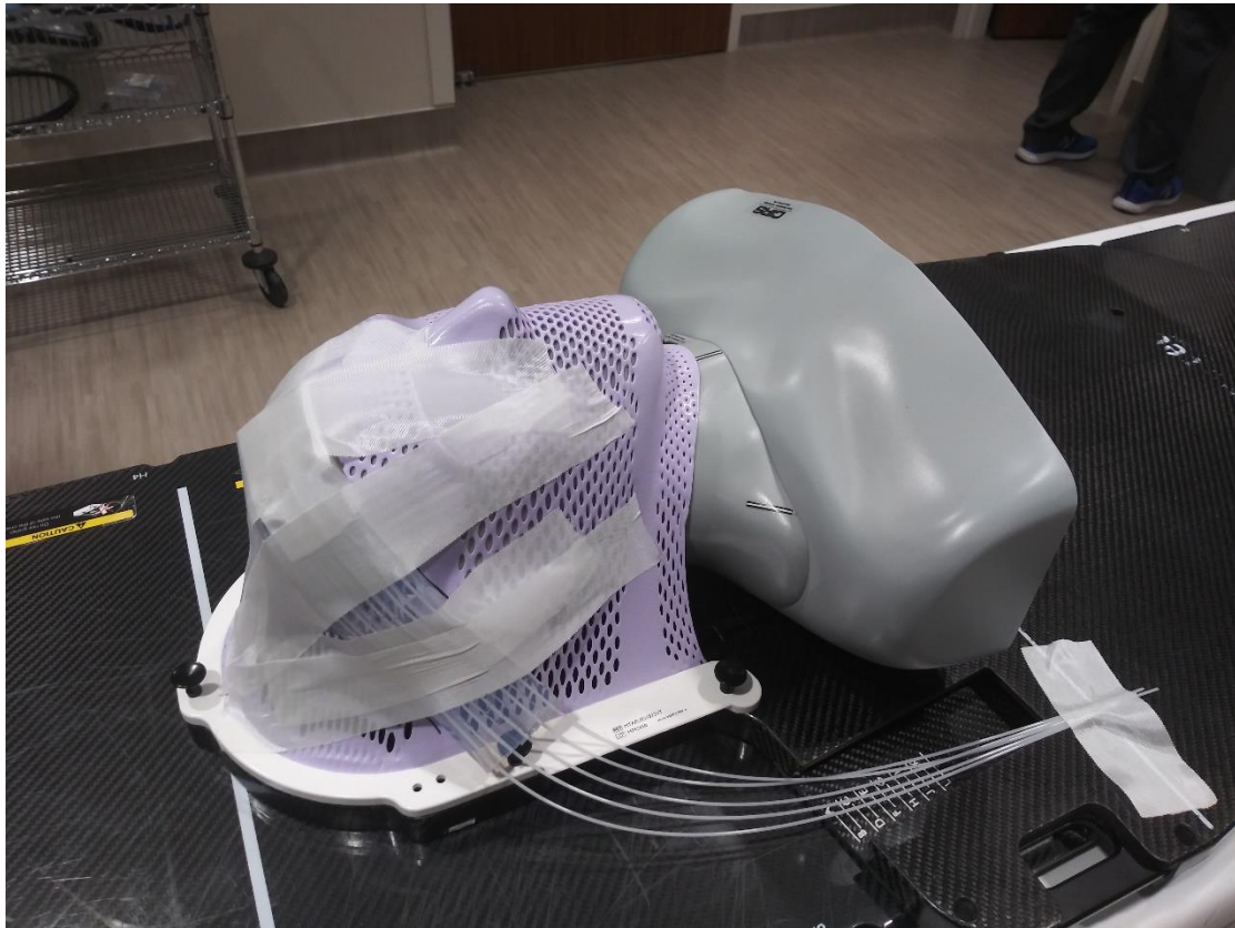
Figure 21: End-to-end test setup on the STEEV phantom.
